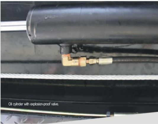
Cylinder with explosion-proof valve
