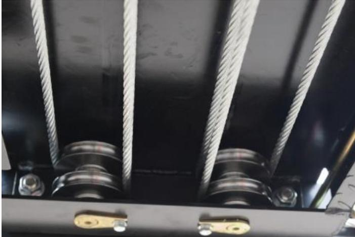
Cables and pulleys under the main runway
